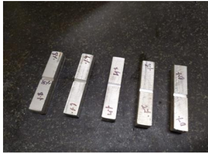
Fig.4 Specimens for Charpy Impact test
