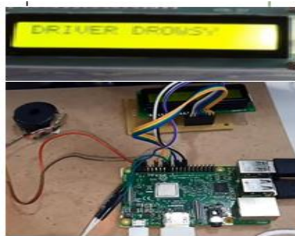
Figure 5: Typical image showing Real time driver's drowsiness detection
