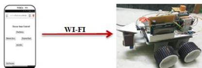
Figure 2 : Smart phone Wi-Fi Controlled the Robot
