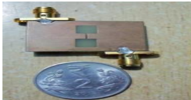
Figure 9: Bottom view after fabrication in MSL
