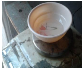
Figure 6: Resin is weighed in weight measuring machine and weight corresponding to the resin is noted.
