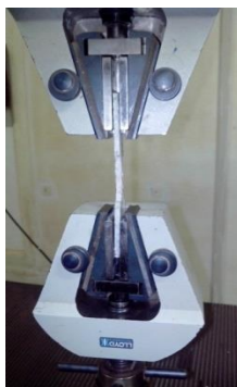
Figure 17: Specimen During Tensile Test (UTM)
