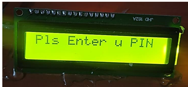
Figure 6: System Asking for Password
