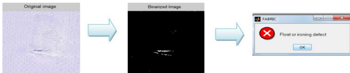
Figure 10: Input , Binarized image and Output window of Float
