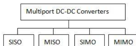
Fig.2. Categorization of multiport DC-DC converter based on number of input and output ports.
