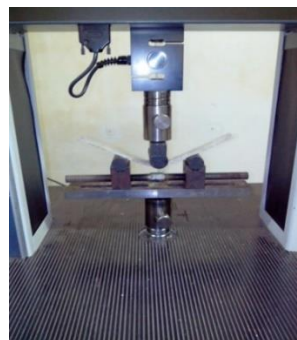
Figure 17: Specimen During Tensile Test (UTM)
