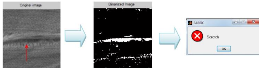
Figure 8 : Input , Binarized image and Output window of Scrath
