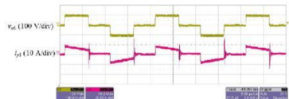
(a) Primary side voltage and current under single - input mode (time base: 5 us/div)
