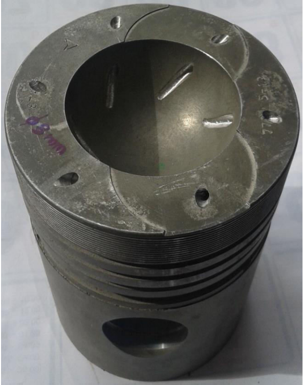
Fig 4.3 Piston 3 - \varnothing 3 \text{ mm} , 6 Elliptical Holes
