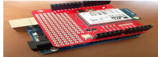
Figure.14. WiFly interfaced with Arduino
