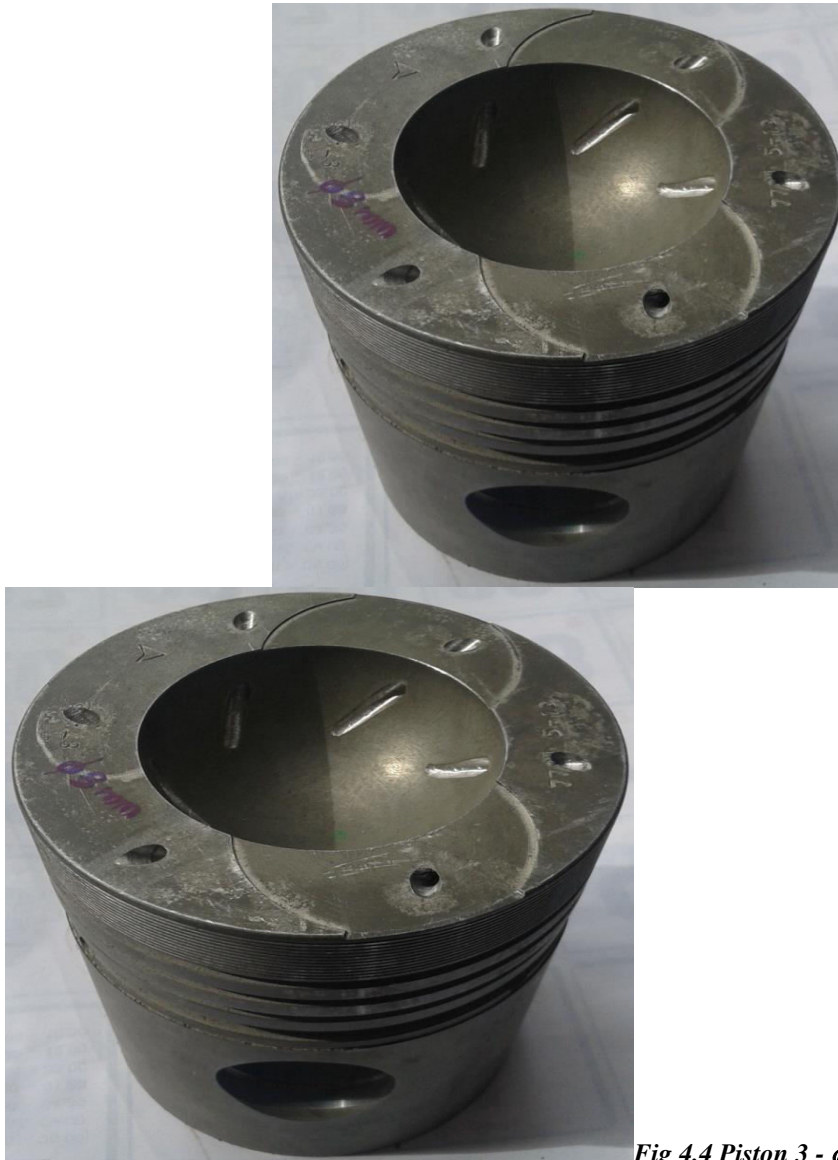
Fig 4.4 Piston 3 - \phi 3mm , 6 Elliptical Holes
