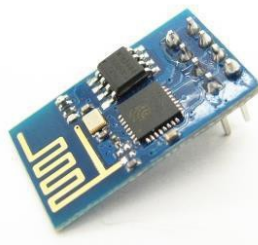
Figure 3. ESP8266-01 WiFi Module
