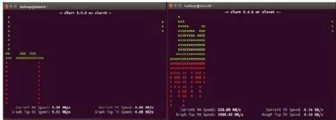
Fig. 8. Traffic Monitoring by Using Slurm Before and During DDoS
