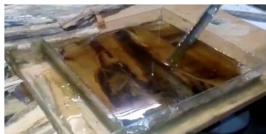
Fig.4. After Resin layer
