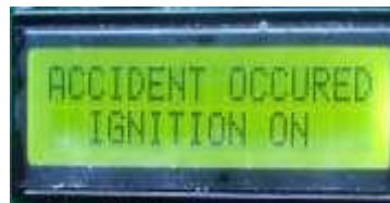
Fig: 2.5. Emergency information Display
