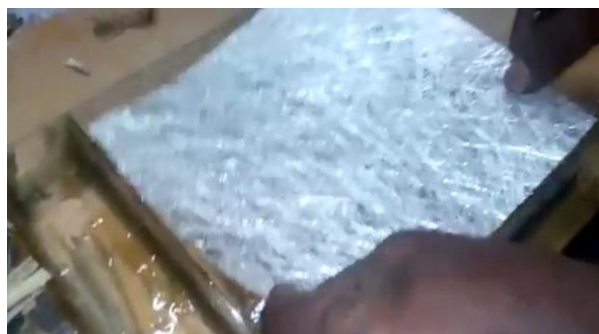
Fig.8.Covered to the layer in Aluminum plate and ready for the compression
