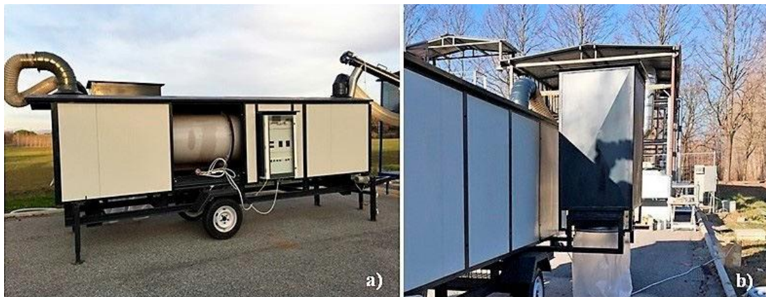
Figure2. Prototype rotary dryer (a); system for recovering dust (b).
