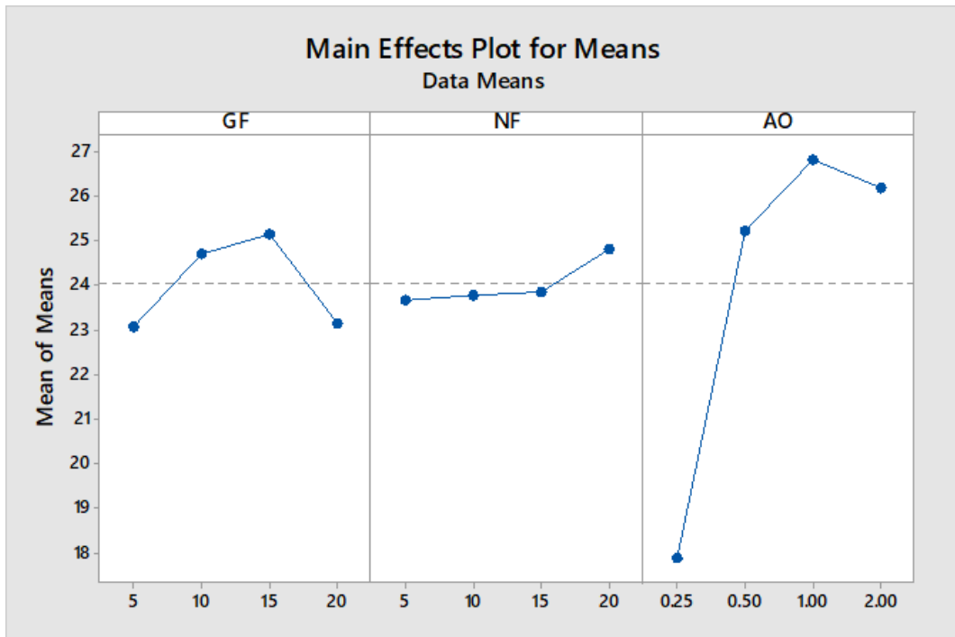
Means value plot of Maximum Tensile stress (Source: Dilip Kumar, Santharaja. M, Ravindra, et al.)
