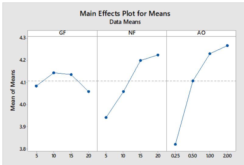
Main effect plots of Young's modulus (Source: Dilip Kumar, Santharaja. M, Ravindra, et al.)
